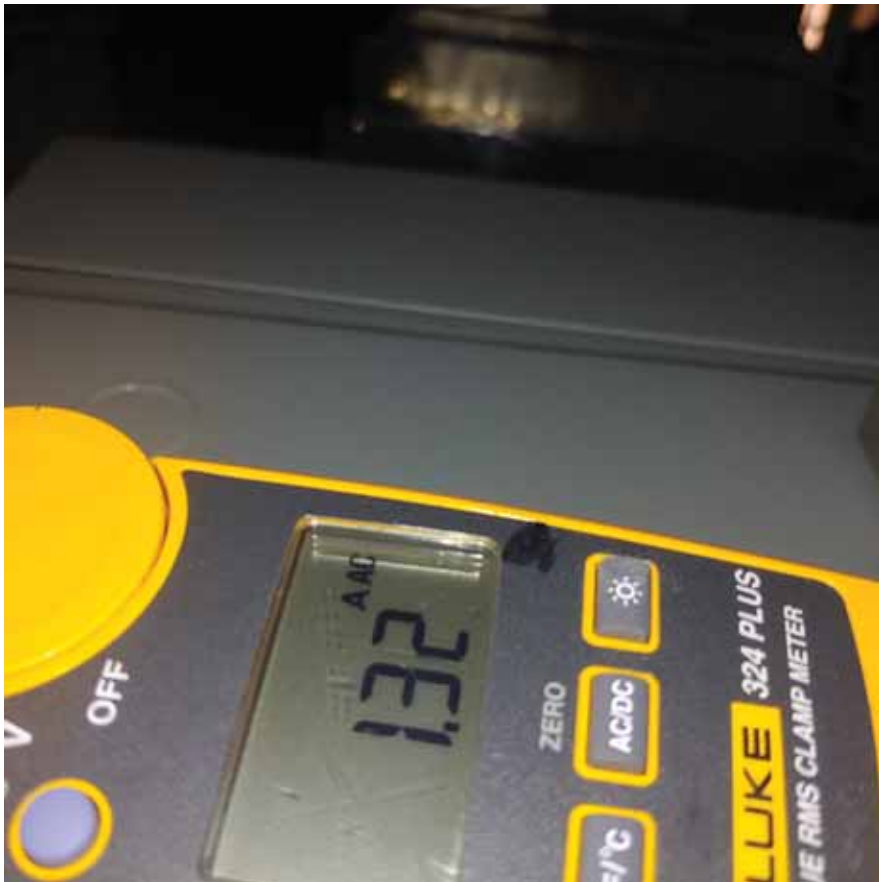
Server/PIC-ahu 1b blower amps.jpg
